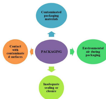
Figure 2: Representation of contamination caused during packaging process
